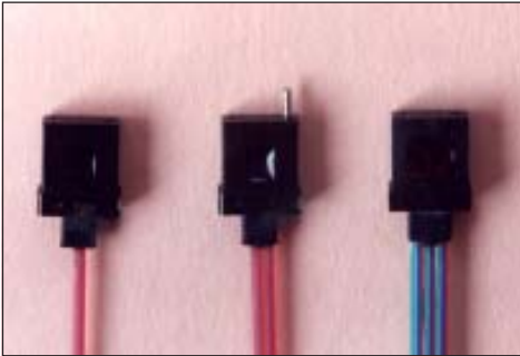
Fig. 8-41 MT-connector for 4-, 8- and 12 fiber ribbon, note the guiding pin in middle connector.
