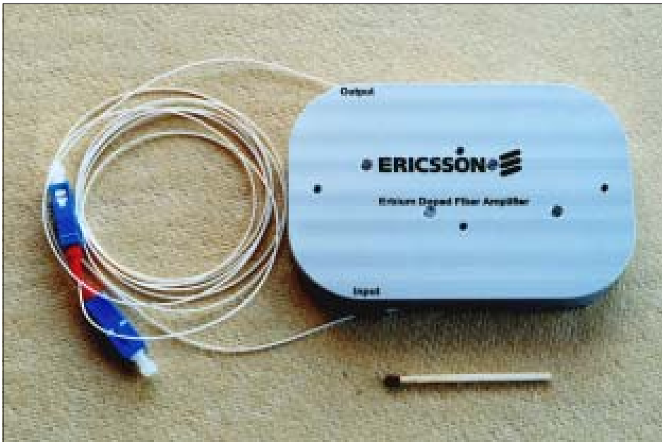
Fig. 12-14 EDFA with a size comparing box of matches.
