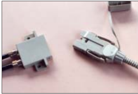
Fig. 8-34 Connector for FDDI network. The connector contains termination for fiber in and fiber out.
