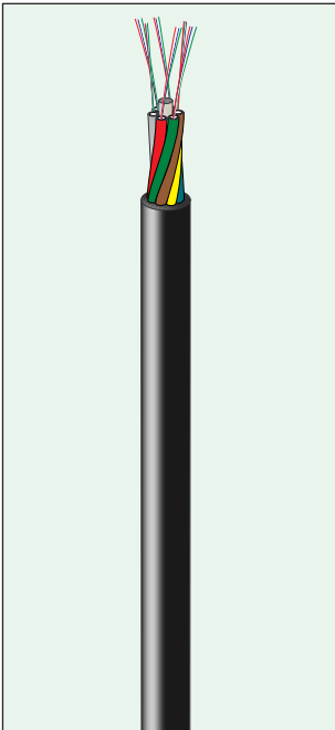
Fig. 5-39 Cable to be wrapped around ground wire or phase line "Skywrap"
