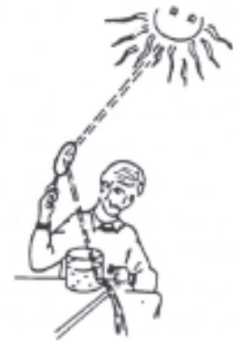
Fig. 1-4 By demonstrating that light could travel along a bent water jet, the principle of optical transmission in light conductors was established.
