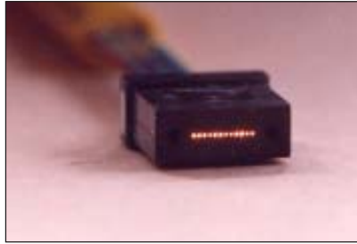
Fig. 8-40 Light coming out of a 12-fiber MT connector
