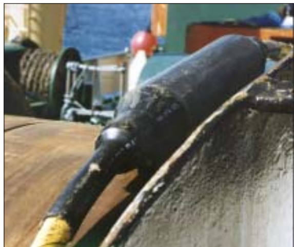
Fig. 11-30 The submarine joint closure SJC 240 ready to go down.
