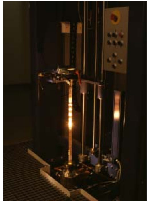
Fig. 3-12 Fiber drawing - top of the tower
