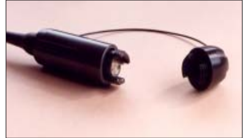
Fig. 8-38 Military field connector utilizing the expanded beam concept.
